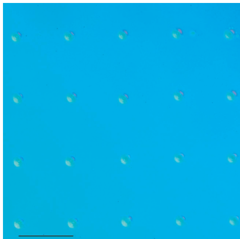
FIGURE 2. Reflective light microscope image of fluid droplets transferred onto a hydrophobized gold surface (scale bar = 25 \mu\text{m} ).
